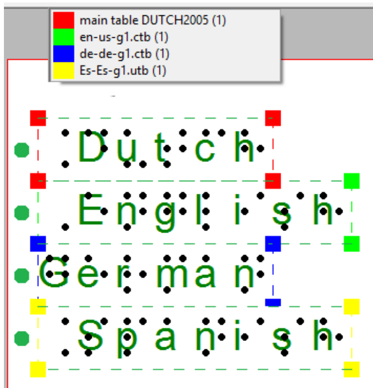
Figure 2. The colours in the legend and text labels signify the used braille tables.
